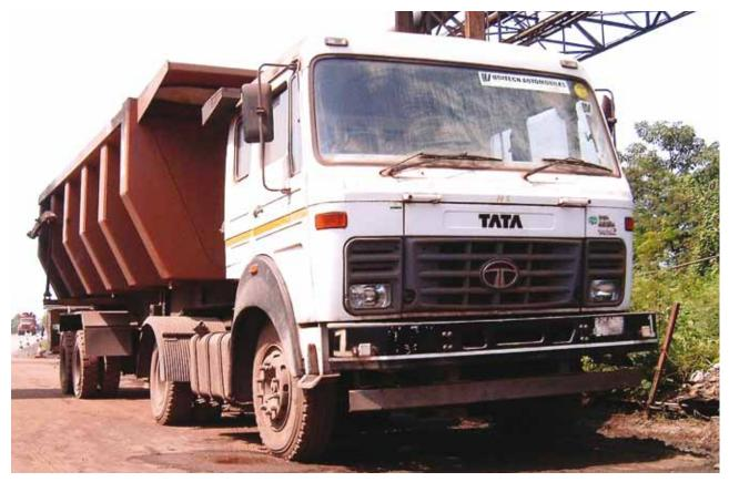
India has developed a reputation for finding out-of-the-box, cost-effective solutions to problems that occur in industry sectors of every kind. When Lloyds Steel Industries required a solution for the disposal of molten slag from furnaces at one of its steel plants, Commercial Engineers and Body Builders Co. (CEBBCO) came up with a trailer fit for the task.
