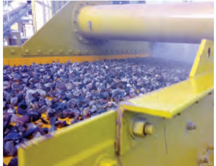
Vibrating Screen in action
